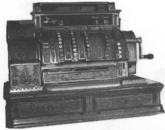
Electrically operated double drawer NCR register. This type was made after 1906
