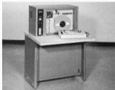
The NCR 735 Magnetic Tape Encoder permits source data to be encoded directly onto magnetic tape — for computer input.
