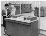
The NCR 420 Optical Reader integrates original entry recordings directly from journal tapes to control EDP processing.
