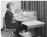
Magnetic Ink Character Recognition (MOCR) imprinting in four fields is provided by the NCR 481 MCR AS-Field Encoder.
