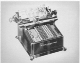
Early type "Batch" Front Machine—items priced in batches after hand-sort by classification of items.
