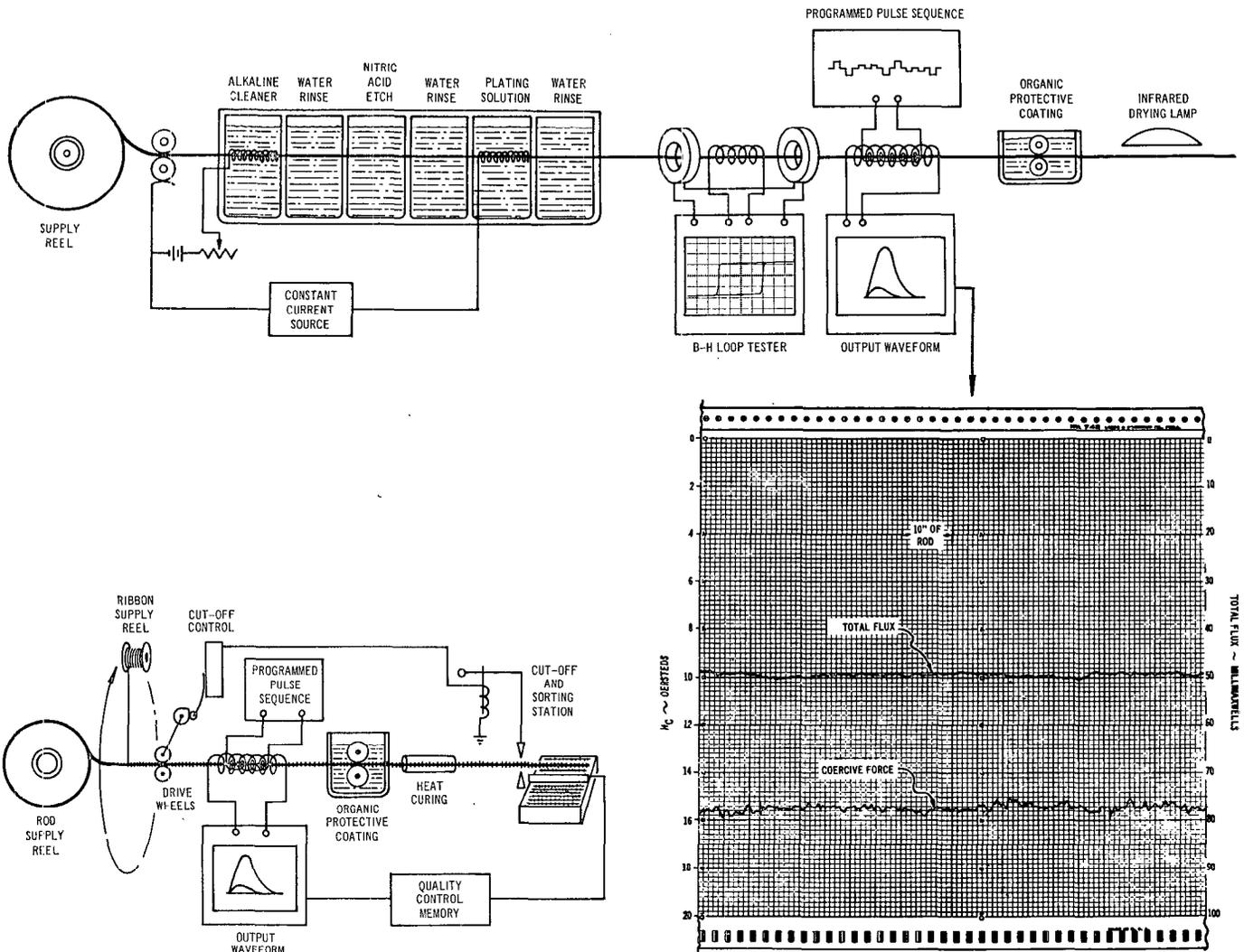
Fig. 3. Automatic coaxial winding line.
